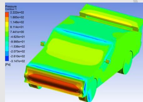
Figure 39: Isometric view pressure contour
