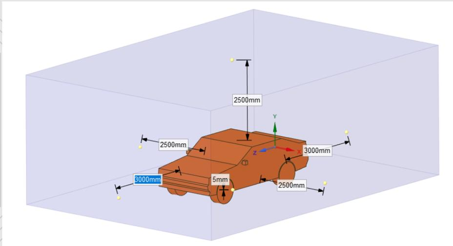
Figure 5: Wind Tunnel conditions
