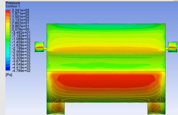
Figure 44: Front view pressure contour
