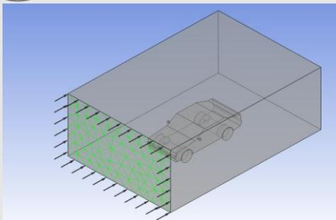
Figure 6: Isometric view of the inlet boundary layer
