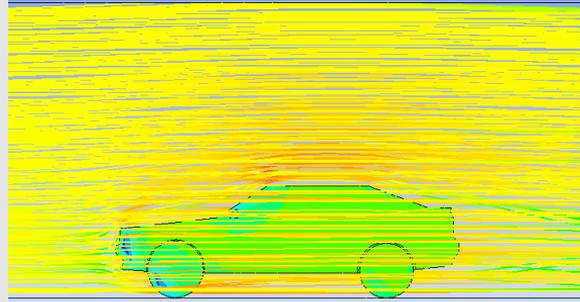
Figure 15: Velocity Streamlines (Side)
