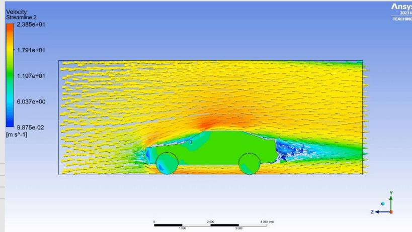
Figure 48: Animation of velocity streamlines for initial design
