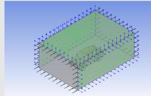
Figure 8: Isometric view of the opening boundary layer
