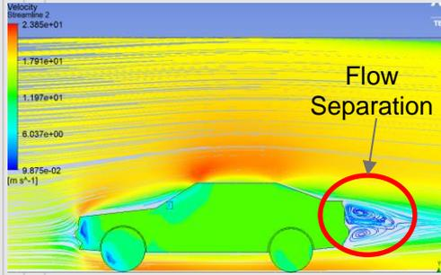
Figure 14: Pressure Contour and Streamlines (Side)
