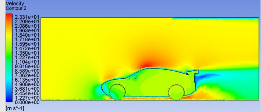
Figure 47: Side view velocity contour
