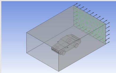
Figure 7: Isometric view of the outlet boundary layer
