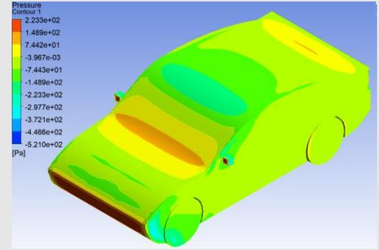
Figure 26: Isometric view pressure contour
