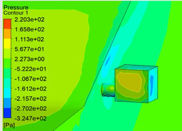
Figure 21: Pressure contour on initial design
