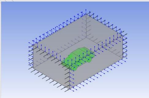
Figure 9: Isometric view of the wall boundary layer
