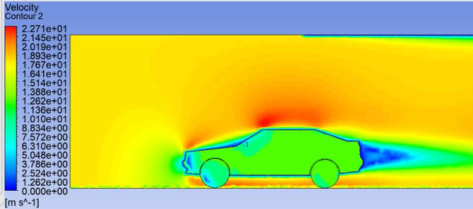
Figure 17: Velocity Contour (Side)
