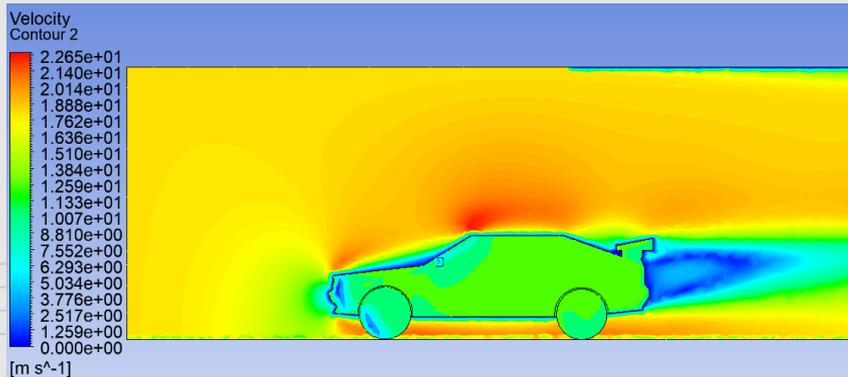
Figure 40: Closeup view of spoiler addition
