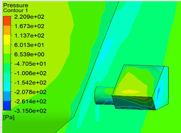
Figure 22: Pressure contour with side mirror improvement
