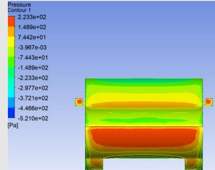
Figure 30: Front view pressure contour
