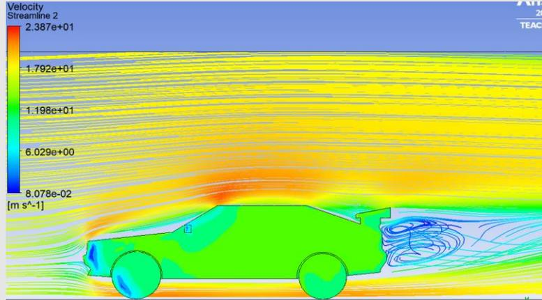
Figure 37: Velocity streamlines side view
